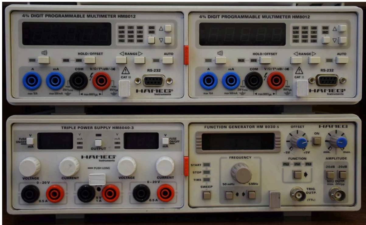
Figure 5.: The electrical instruments at the lab TA105, without the oscilloscopes
