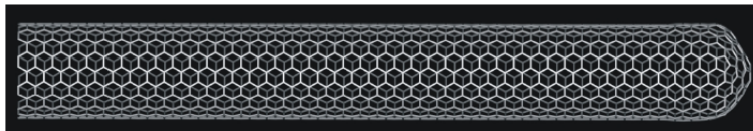
Fig. 1: Computer model of a single-walled carbon nanotube.
