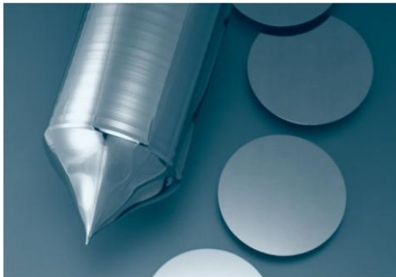
Fig. 13 300 mm (12 in.) ingot and polished silicon wafers
