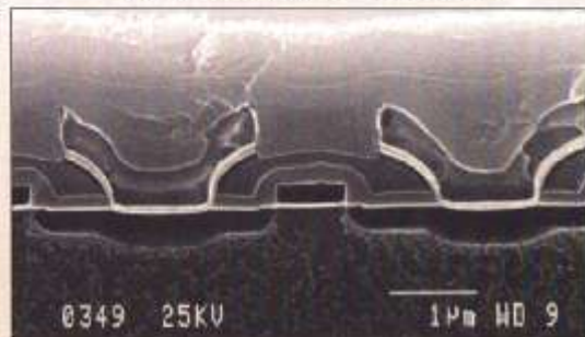
0.8 μm CMOS transistor cross-section
