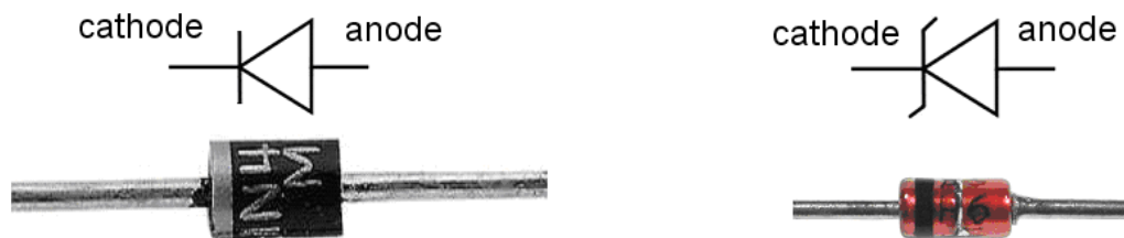
Figure 1.1: Connection of 1N4007 Si diode (left), and of the Zener-diode (right)
