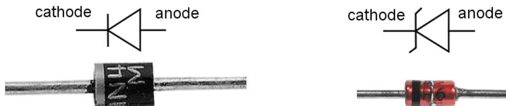
Figure 2.1: Connection of 1N4007 Si diode (left), and of the Zener-diode (right)
