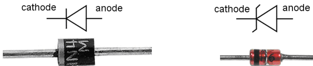
Figure 1: Connection of 1N4007 Si diode (left), and of the Zener-diode (right)
