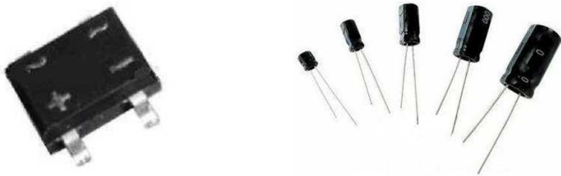
Figure 7. Left: Integrated Graetz bridge; Right: Electrolytical Capacitors
