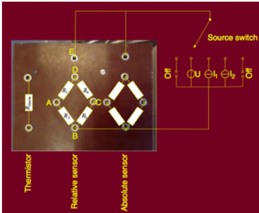
Figure 3: Test setup top side and the circuitry behind
