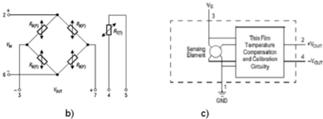
Figure 1: b) internal structure of a relative and an absolute sensor;
