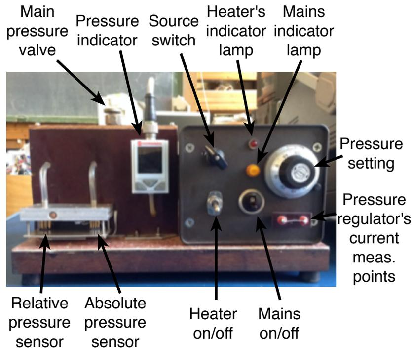
Figure 2: Test setup front side
